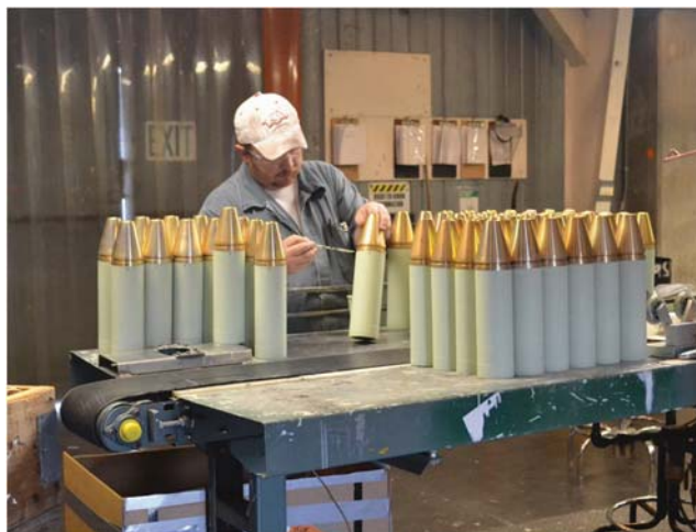
Pine Bluff Arsenal employee seals M819 81mm red phosphorus smoke mortars on a Load Pack and Assemble production line
