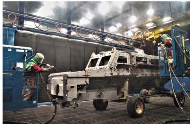
Workers at Letterkenny Army Depot clean a frame before beginning overhaul work
